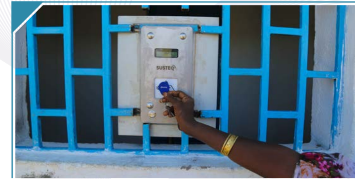
Figure 2: A community member using an automated prepaid payment system at Kargi water Kiosk in Marsabit County
